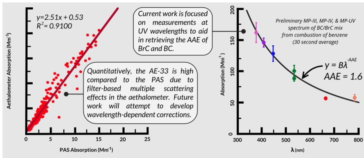
Figure 6: Comparison of the Magee Scientific AE-33 7-wavelength aethalometer to MP-IV at 660/662 nm with ambient aerosols in Athens, GA (left) and the UV-visible spectrum of a mix of black and brown carbon generated in the lab of Dr. Rawad Saleh and obtained with MP-IV, MP-UV, and MP-III simultaneously (right).
