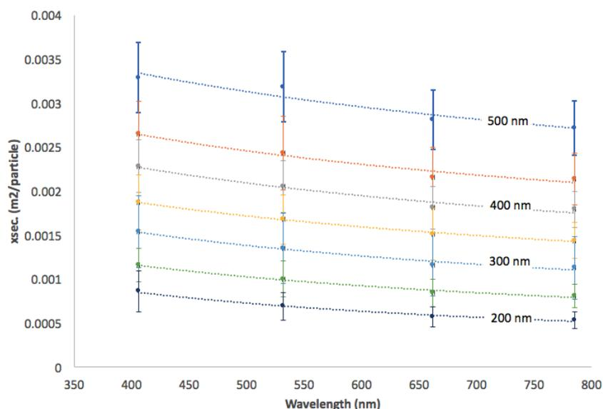
Figure 3: Preliminary carbon black spectra acquired with MP-IV for NIST. Various colors are different sizes selected with a differential mobility analyzer, ranging from 200 to 500 nm in 50 nm increments. Dashed lines are power law fits (Equation 1) to the data.
