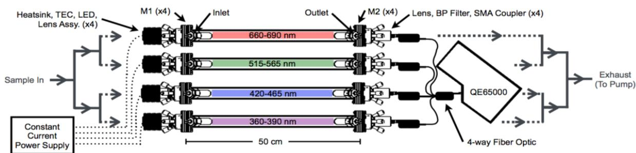
Figure 1: A schematic of the original 4-channel BBCES constructed during the early stages of my thesis work. M = mirror, TEC = thermoelectric cooler, LED = light emitting diode, BP Filter = bandpass filter.
