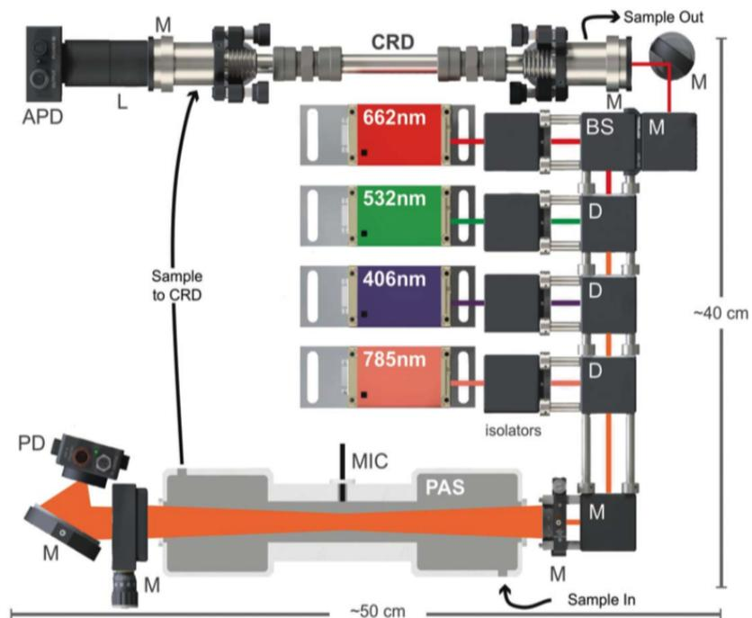
Figure 2: A diagram of the MultiPAS system, showing the 4 channel version. M = mirror, CRD = cavity ringdown, D = dichroic mirror, PAS = photoacoustic cell, mic = microphone, (A)PD = (avalanch) photodiode. Reprinted from Fischer and Smith (2017)<sup>20</sup>
