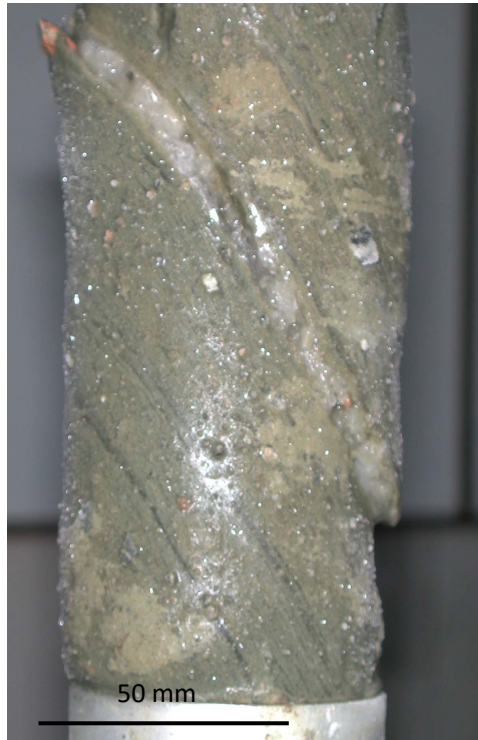
Figure 7. Result of a triaxial test of a sample of the laminated subfacies showing failure localized to an ice-rich layer in the laminated subfacies. This test was undertaken with the sample in an air-filled pressure vessel maintained at 200kPa and -18°C for the duration of the 12 hr test.
