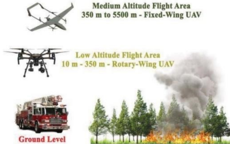
Figure 1. The main part of the platform for early forest fire detection with use of fixed wing and rotary wing UAVs
