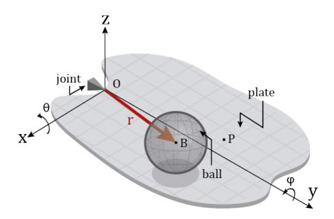
Figure 1: Group of coordinates considered to describe ball and plate dynamics. Point O represents the origin of rotating and non-rotating frame located near to the joint. Point P is the center of mass of the plate. Point B is the center of mass of the ball.
