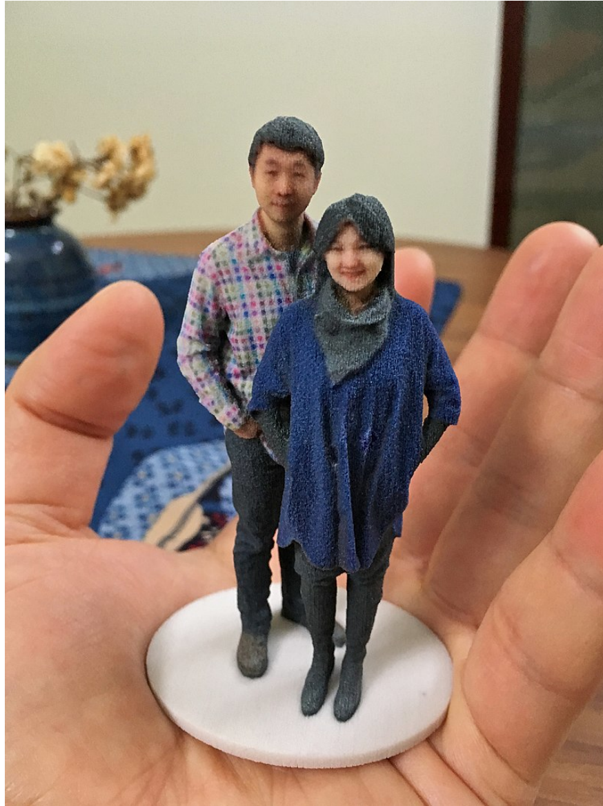
Figure 5: A 3D selfie in 1:20 scale printed by Shapeways using gypsum-based printing. Źródło: UEK materiały
