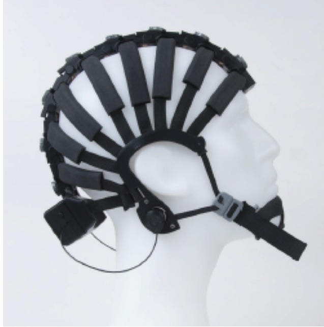
Figure 2: The dry-EEG system HD-72 model developed by Cognionics Inc. (San Diego, USA).
