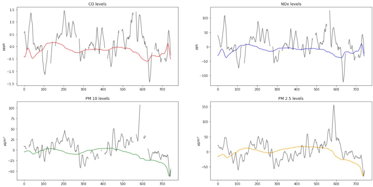
Figure 6: Change point detection curve fitted through data for a one month period
