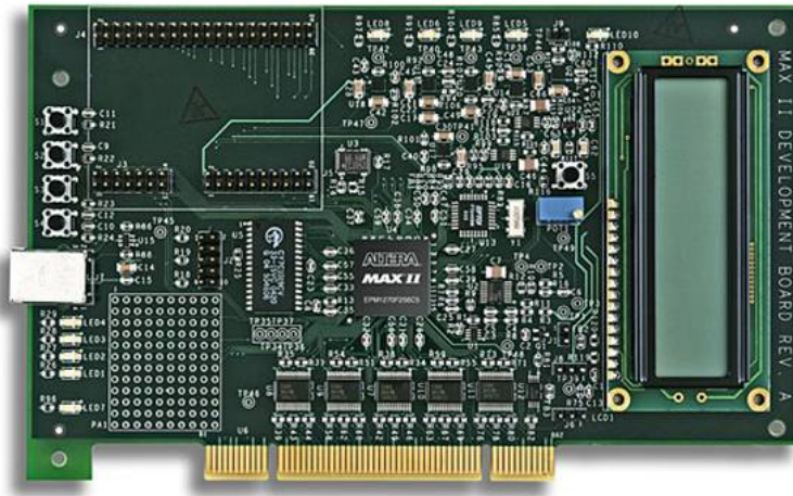
Figure 2. Altera Max II Development Board In this board, a EPM1270 FPGA is described the PIC used in the FPAA prototyping board to adapt the frequency response for the Front-End scheme.
