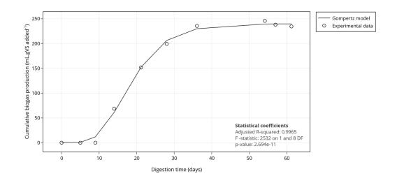
Figure 6: Fitting of Gompertz model to cumulative biogas production data obtained from Weaners wastewater digestion.
