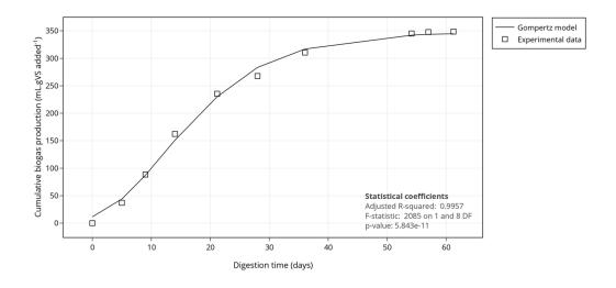
Figure 5: Fitting of Gompertz model to cumulative biogas production data obtained from Fattening wastewater digestion.
