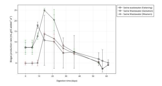
Figure 2: Biogas production rate (ml .~gVS added  $^{-1}$   $.~d^{-1})$  of fattening, gestation and weaners wastewater.
