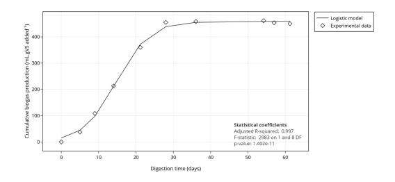
Figure 4: Fitting of logistic model to cumulative biogas production data obtained from Gestation wastewater digestion.
