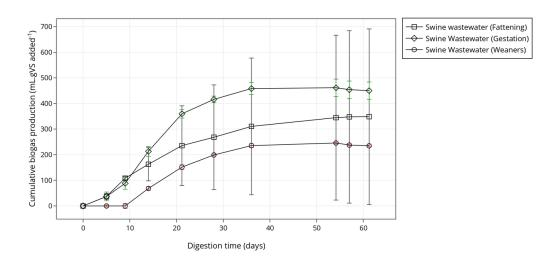
Figure 1: Cumulative biogas production (ml . gVS added<sup>-1</sup>) of fattening, gestation and weaners wastewater.
