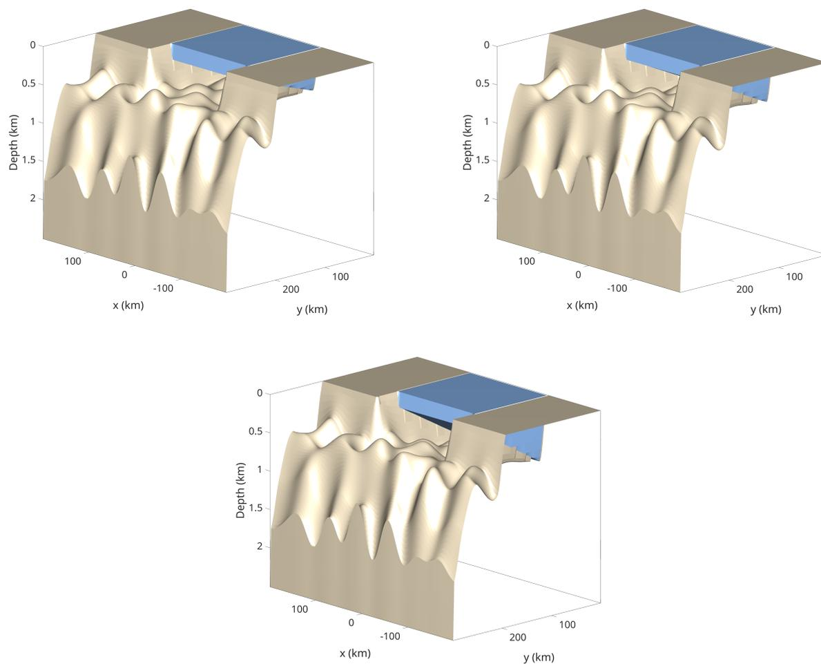
**Figure S8.** Model geometry of simulations with varying bed slopes. On the top left, a simulation with a continental shelf 300 m deeper than the grounding line (s300). On the top right, a simulation with a continental shelf 150 m deeper than the grounding line (s150). On the bottom, a simulation with a continental shelf 0 m deeper than the grounding line (s0).
