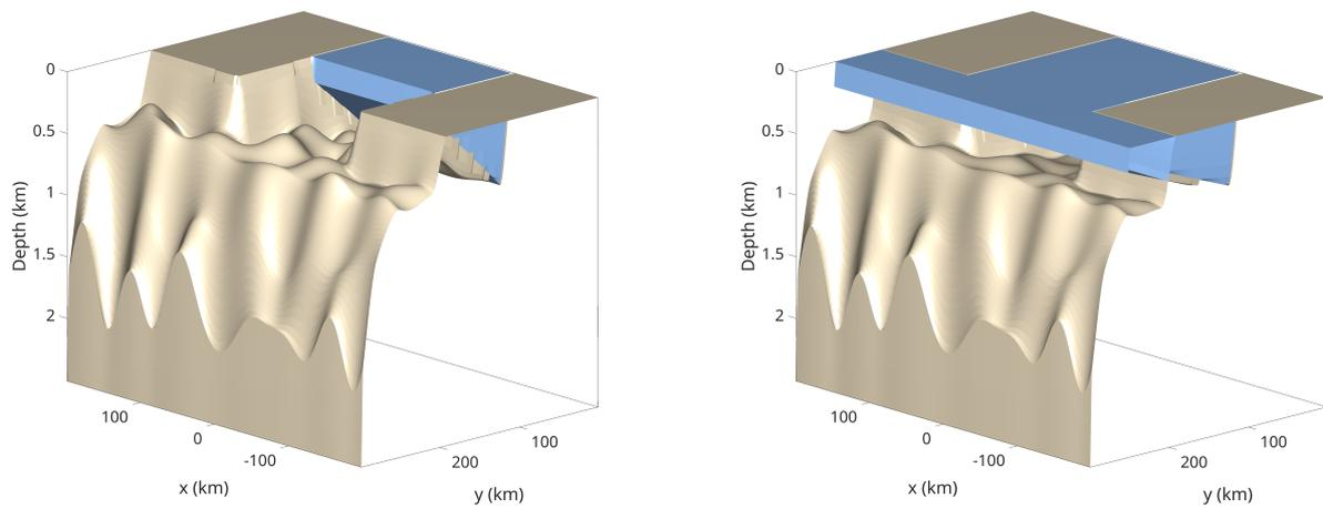
**Figure S6.** Model geometry of simulations with varying ice shelf extents. On the left, a simulation with an icefront of 100 km (y100). On the right, a simulation with an icefront of 250 km (y250)
