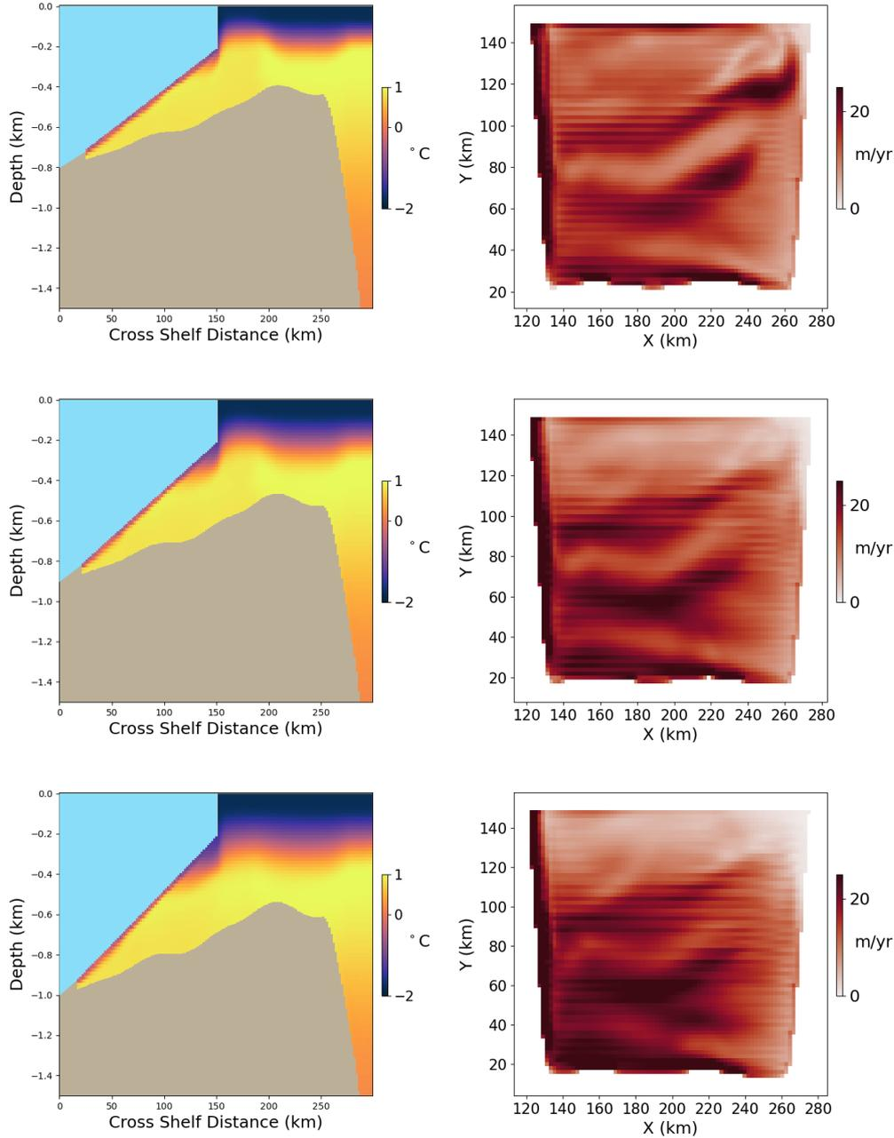
**Figure S12.** Meridional cross sections of time-average potential temperature (left column) and maps of time-average ice shelf melt in m/yr (right column) from high thermocline model simulations with varying shelf depths. At the top, a simulation with a depth of 500 m (d500). In the middle, a simulation with a shelf depth of 600 m (d600). On the bottom, a simulation with a shelf depth of 700 m (d700).
