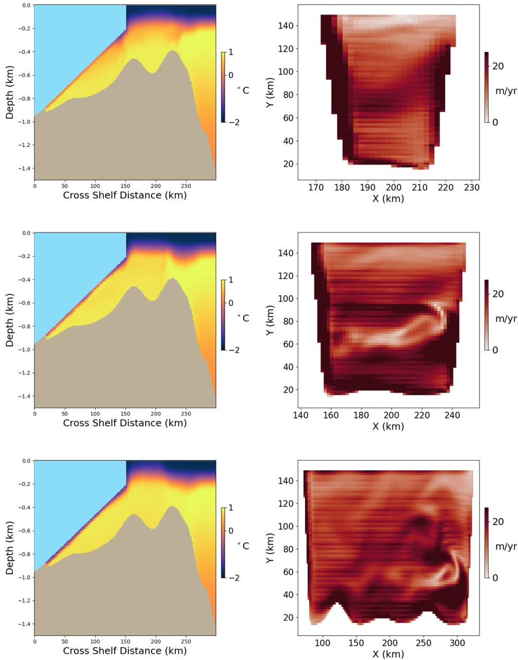
**Figure S14.** Meridional cross sections of time-average potential temperature (left column) and maps of time-average ice shelf melt in m/yr (right column) from high thermocline model simulations with varying cavity widths. On the top, a simulation with a continental shelf 50 km wide (w50). In the middle, a simulation with a continental shelf 100 km wide (w100). On the bottom, a simulation with a continental shelf 250 km wide (w250).
