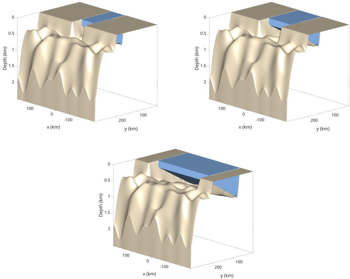
**Figure S9.** Model geometry of simulations with varying cavity widths. On the top left, a simulation with a continental shelf 50 km wide (w50). On the top right, a simulation with a continental shelf 100 km wide (w100). On the bottom, a simulation with a continental shelf 250 km wide (w250).
