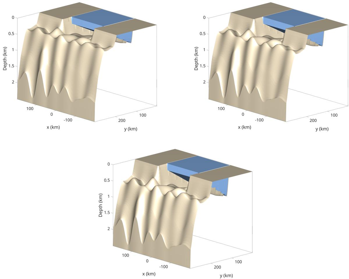
**Figure S7.** Model geometry of simulations with varying shelf depths. On the top left, a simulation with a depth of 500 m (d500). On the top right, a simulation with a shelf depth of 600 m (d600). On the bottom, a simulation with a shelf depth of 700 m (d700).
