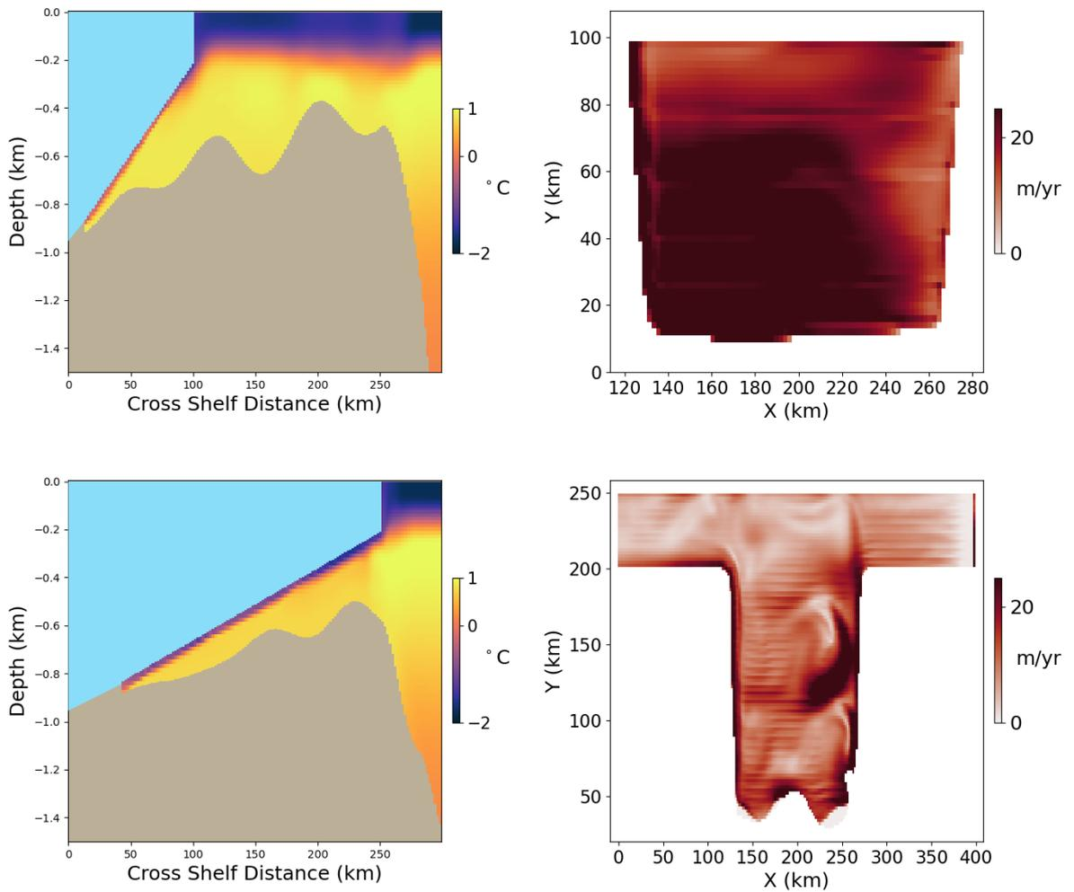
**Figure S11.** Meridional cross sections of time-average potential temperature (left column) and maps of time-average ice shelf melt in m/yr (right column) from high thermocline model simulations with varying ice shelf extent. At the top a simulation with an icefront of 100 km (y100). On the bottom, a simulation with an icefront of 250 km (y250)
