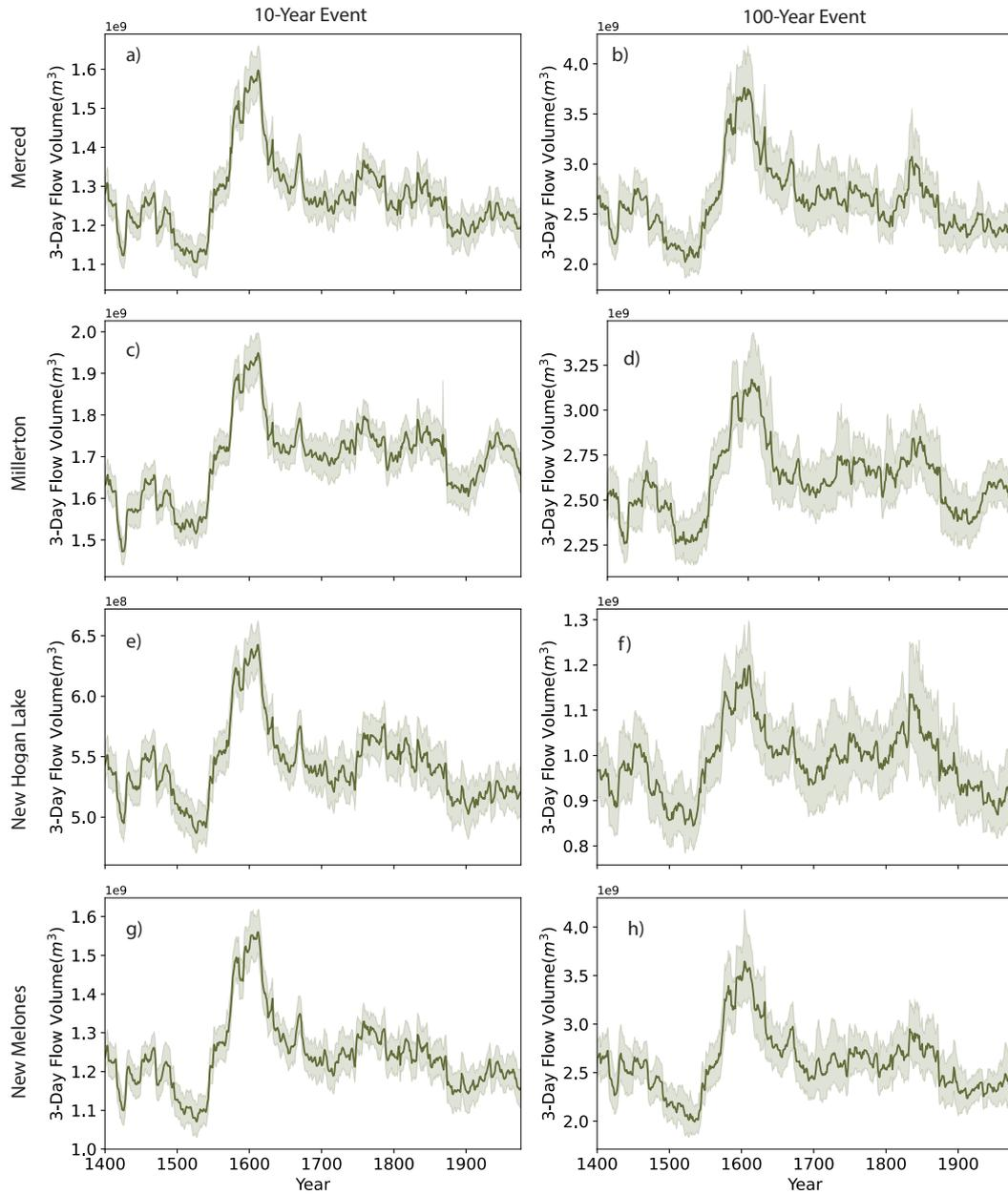
**Figure S10.** Three-day annual maxima associated with the 10-year return period event and 100-year return period event for remaining four gauged locations. calculated in 30-year moving windows and across the time period from 1400-2017. The dark green line represents the mean flooding return levels and the shading represents the 5<sup>th</sup> and 95<sup>th</sup> percentile bounds.
