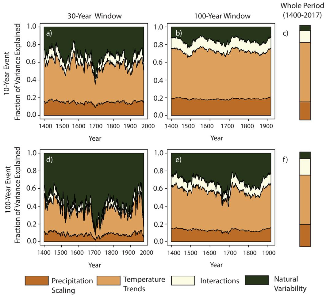
**Figure S13.** A decomposition of the key drivers of variance in the flood metrics for the Merced Falls gauge in the Merced River Basin for an a,d) 30-year window b,e) 100-year window and c,f) a 600-year window.
