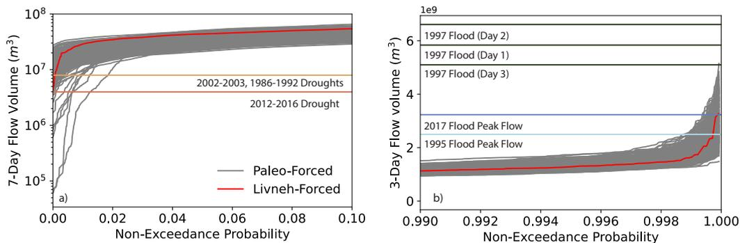
**Figure 4.** a) 7-day and b) 3-day flow volumes at the Don Pedro gauge in the Tuolumne Basin derived from the paleo-informed streamflow ensembles compared to the Livneh-forced generator over the modern period. Key events from the observed record are shown as colored lines. Each grey line represents sorted volumes for each year in 30-year chunks of the paleo-reconstruction across all 50 ensemble members.
