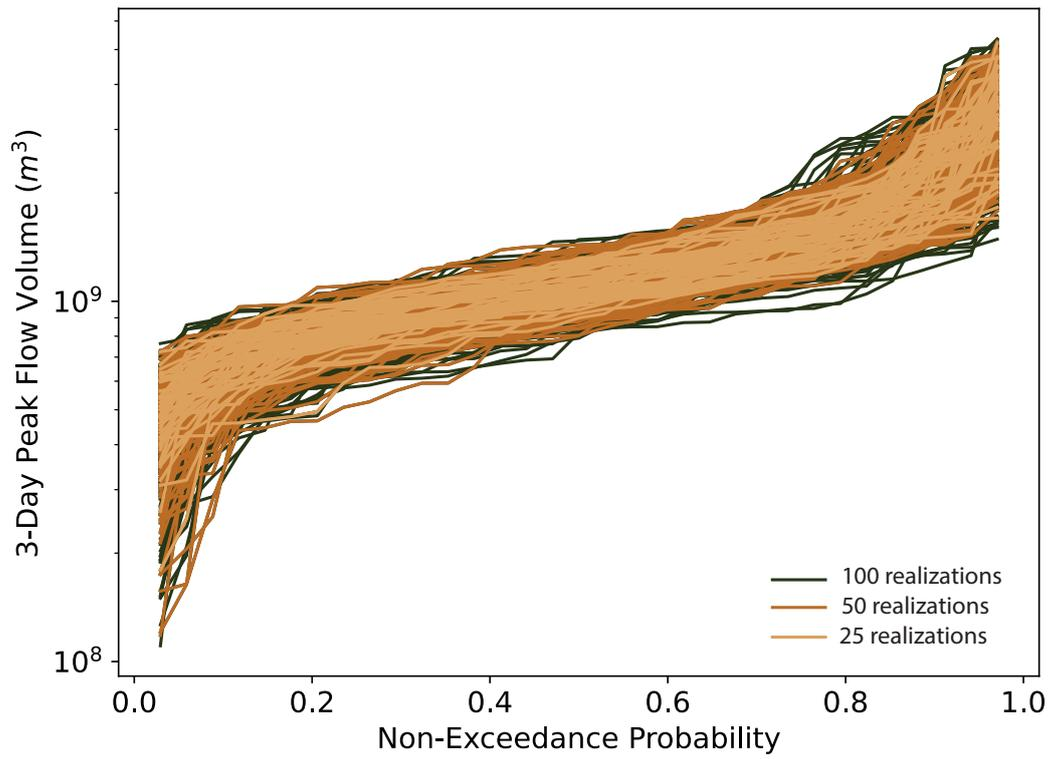
**Figure S1.** Flow duration curves of 3-day peak flow corresponding to different ensemble sizes. Each line corresponds to 30-year chunks of the 600-year record.
