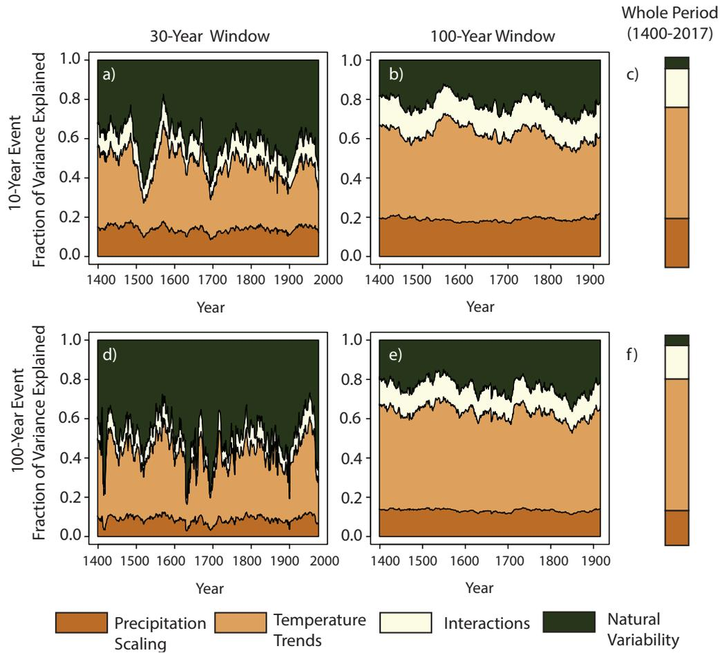
**Figure S14.** A decomposition of the key drivers of variance in the flood metrics for the Millerton Lake gauge in the San Joaquin Basin for an a,d) 30-year window b,e) 100-year window and c,f) a 600-year window.
