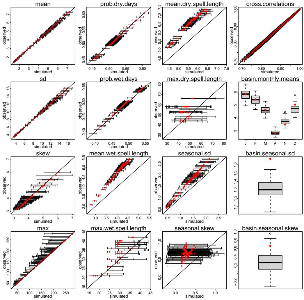
**Figure S3.** Observed vs. simulated characteristics of daily precipitation in the Tuolumne Basin. For at-site characteristics (180 grid cells), the 95% range for simulated statistics across the 50 ensemble members is shown with whiskers. For basin-averaged statistics, the distribution of simulated statistics is shown as a boxplot along with the observed value.
