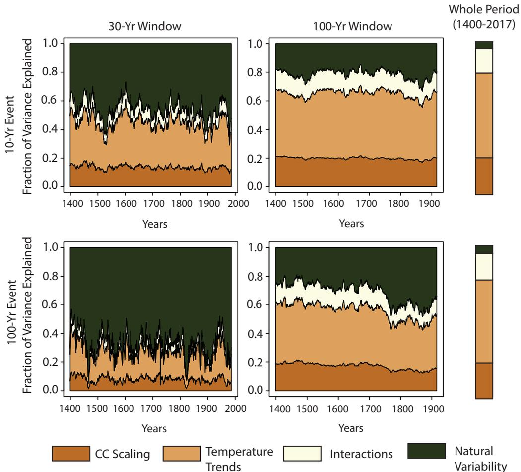
**Figure 11.** A decomposition of the key drivers of variance in the flood metrics for the Don Pedro gauge in the Tuolumne River Basin for an a,d) 30-year time horizon b,e) 100-year time horizon and c,f) a 617-year time horizon.
