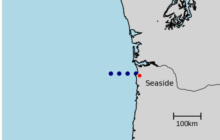
Figure 15: A minimal arrangement of buoys tested with aims to achieve similarly accurate results as a tight grid. Chosen based on sensitivity measurements (Figure 4.35) are four buoys spaced 27 km apart extending out to sea from the site of interest.
