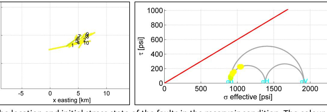
The location and initial stress state of the faults in the reservoir condition. The colour represents the pore pressure required for the fault to slip in Mohr-Coulomb failure
