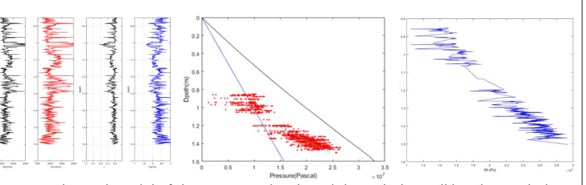
1D geomechanical model of the reservoir developed through the well log data including Poisson's ratio, pore pressure, and horizontal stress.
