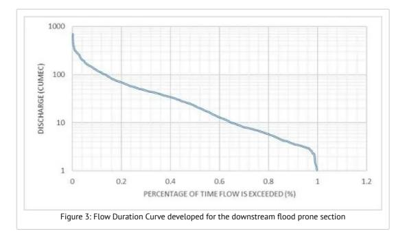
• Figure 3 shows the FDC curve developed at the downstream flood prone section. The FDC was prepared using the available daily streamflow data of the downstream section from the year 2003-2012.
