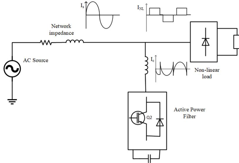
FIGURE 1 Schematic representation of the PCC-connected shunt active power filter
