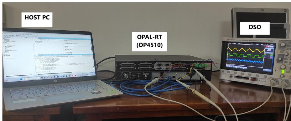
FIGURE 12 Real Time experimental setup using OP4510
