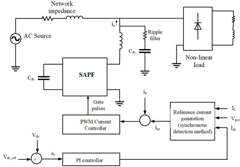
FIGURE 2 Model for simulating the proposed method.
