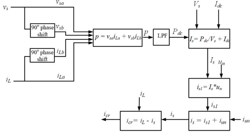
FIGURE 3 Calculation of reference current using proposed method
