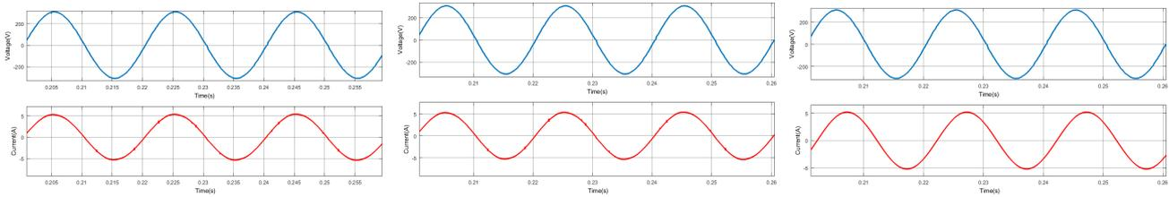
FIGURE 7 Waveforms at consumer ends for case 5 with APF when source voltage is sinusoidal.
