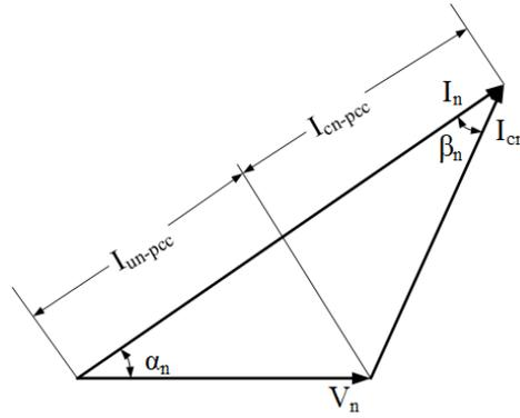
FIGURE 4 Phasor representation of the  $n^{\text{th}}$  harmonic quantities.
