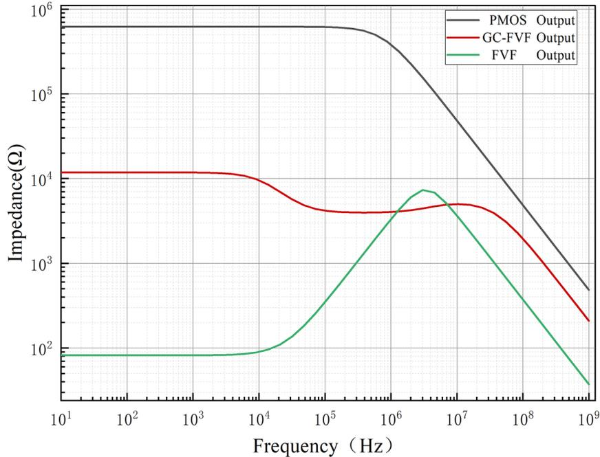
**Fig. 4.** Output impedance characteristic of PMOS, GC-FVF and FVF topologies.
