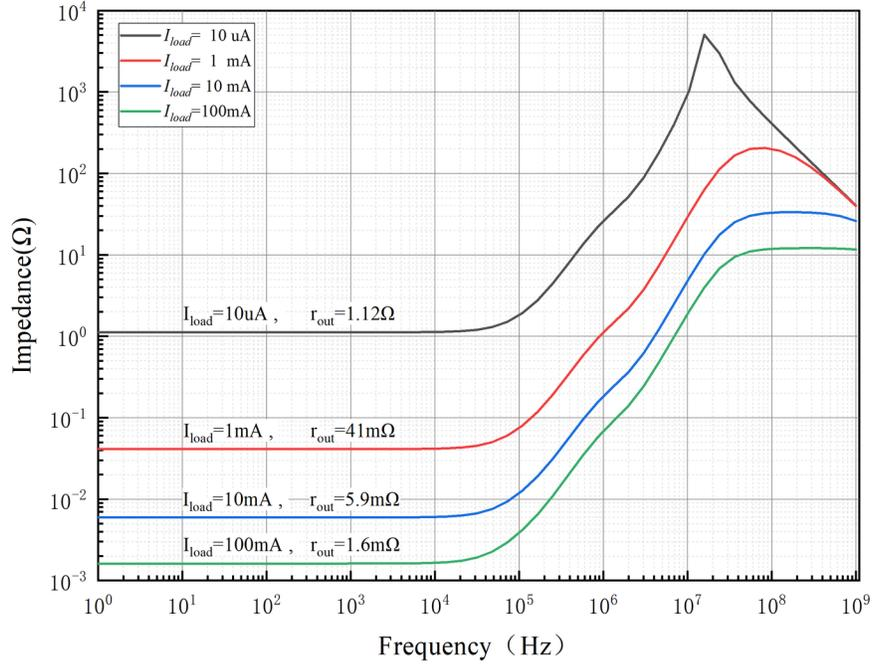
**Fig. 5.** Output impedance characteristic of the proposed GC-FVF LDO.
