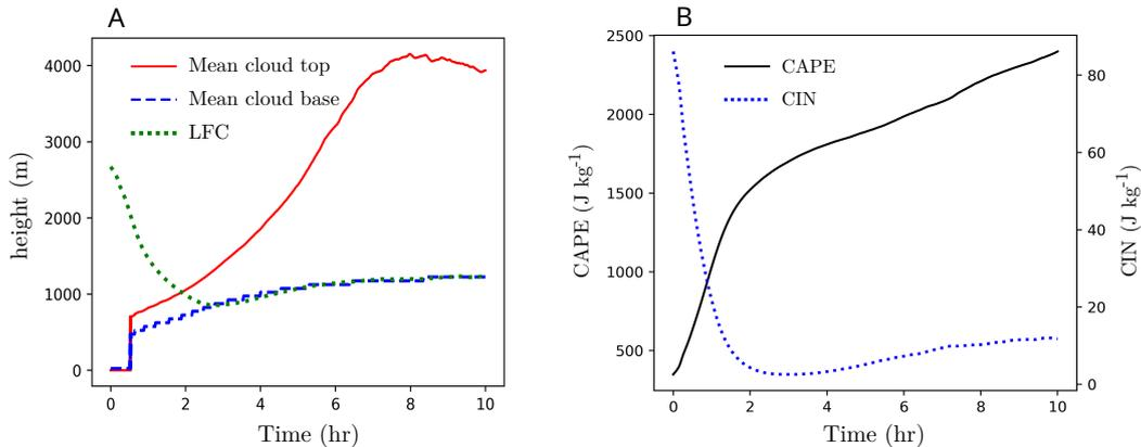
**Figure 5.** Shallow-to-deep transition in the idealized LBA case. (A) Time series of mean cloud top (red solid line), mean cloud base (blue dashed line), and LFC (green dotted line). (B) Time series of CAPE (black solid line) and CIN (blue dotted line).
