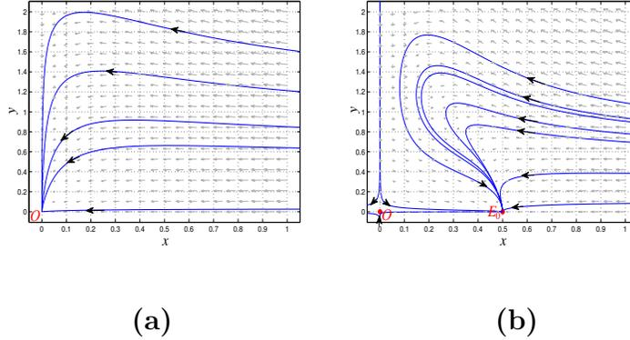
Figure 1: Phase portraits of boundary equilibria for system (6) at  $\alpha_1 = 0.3$ ,  $\alpha_2 = 0.9$ ,  $h_2 = 0.2$ ,  $\gamma = 0.03$ . (a)  $O(0,0)$  is a stable node for  $h_1 = 1.3$ . (b)  $O(0,0)$  is unstable and  $E_0(1 - h_1, 0)$  is stable for  $h_1 = 0.5$ .
