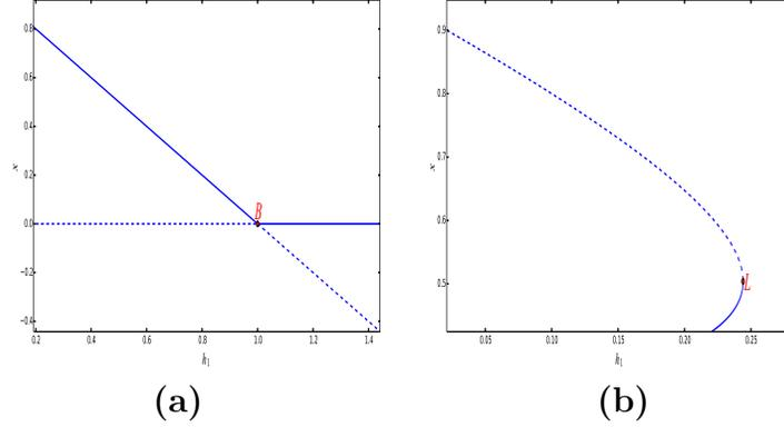
Figure 5: Bifurcation diagrams for system (6) with respect to the bifurcation parameter  $h_1$  under condition (27). **(a)** Transcritical bifurcation at  $O(0,0)$  for  $h_1 = h_1^{TC} = 1$ . **(b)** Saddle-node bifurcation at  $E_1(0.503967, 0.848173)$  for  $h_1 = h_1^{SN} = 0.244047$ .
