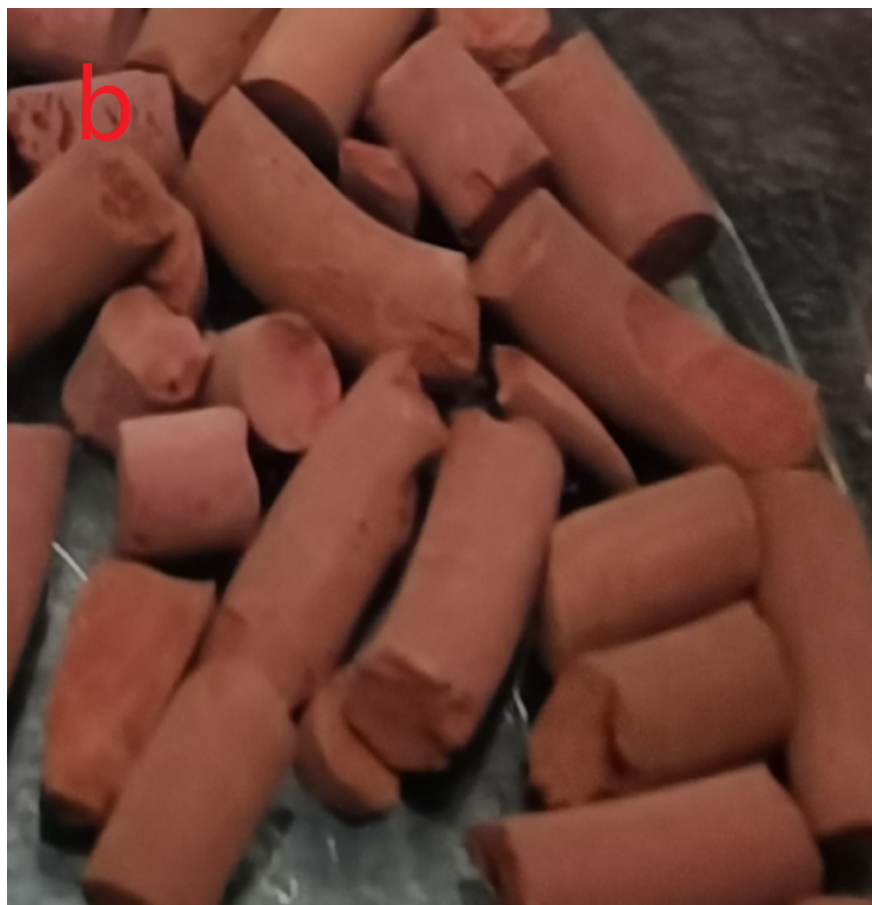
Figure 4 Color of (a) silicalite-1 and (b) silicalite-1 after iodine adsorption
