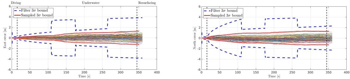
Figure 6: East and North position estimation errors versus their  $3\sigma$  bounds obtained from 100 simulation analysis with the SLAM algorithm. The  $\sigma$  values are computed as the square-root of the corresponding diagonal element of the estimated covariance matrix.
