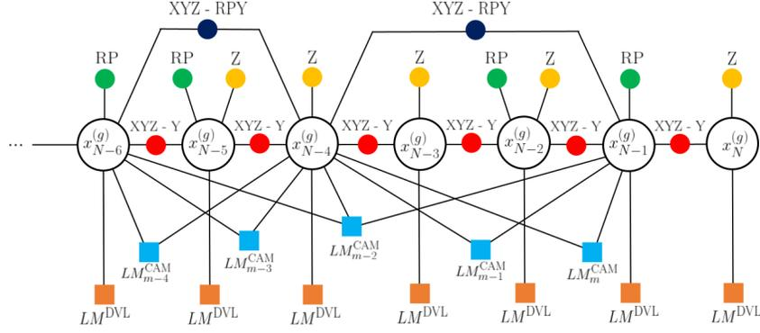
Figure 3: Last nodes of the factor graph  $g$  constrained with vision-based landmarks and all the onboard sensors.
