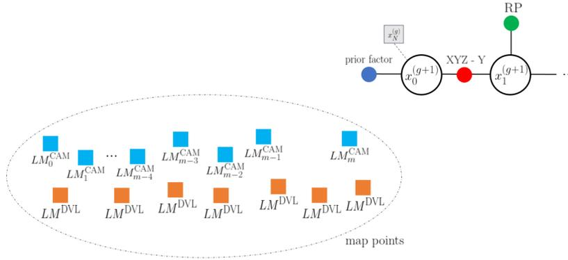
Figure 5: First nodes of the factor graph  $g + 1$  after the employment of the global reset procedure. The values in the grey boxes represent the corresponding states taken from the previous factor graph  $g$  and transferred to the actual graph  $g + 1$ .
