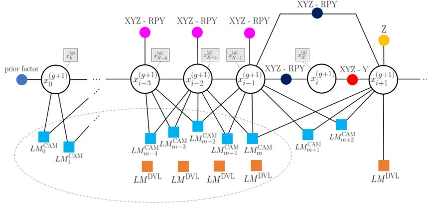
Figure 4: First nodes of the factor graph  $g + 1$  after the employment of the keyframe reset procedure. The values in the grey boxes represent the corresponding states taken from the previous factor graph  $g$  and transferred to the actual graph  $g + 1$ .
