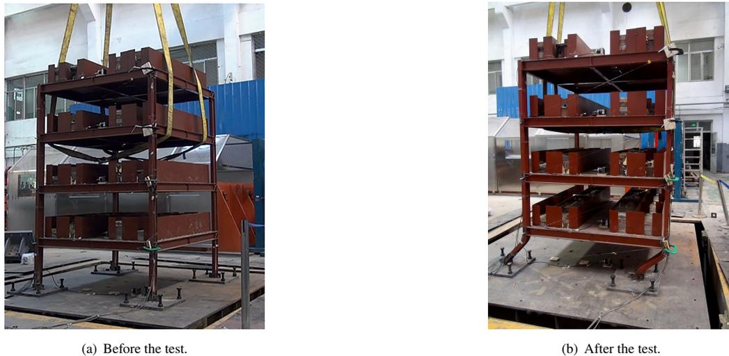
**FIGURE 3** Red four-layer RC frame, yellow rope providing backup support but no direct contact and earthquake simulation shaking table.
