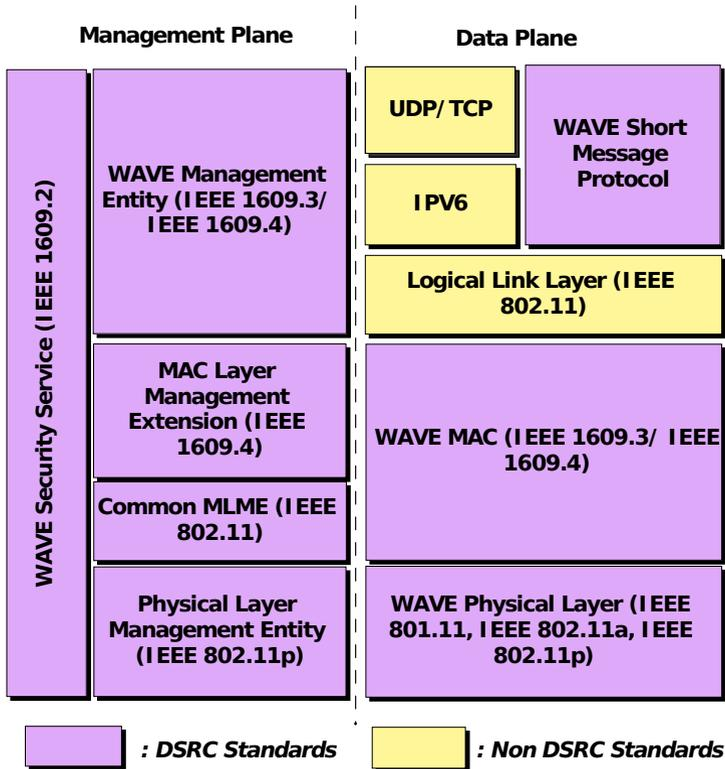
Fig. 3 A WAVE protocol stack
