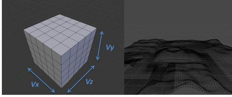
**Figure 3** Subdivision of the 3D space into cells.
