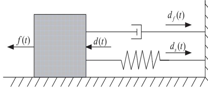
**Figure 2** Schematic diagram of the mass-spring-damper model.
