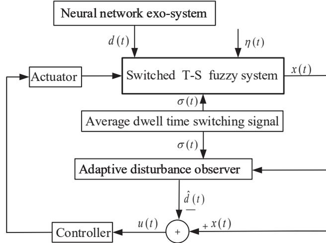
**Figure 1** Configuration of the AADS control.
