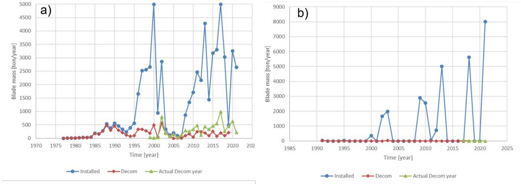
**FIGURE 6** Installed and decommissioned blade mass of a) onshore and b) offshore wind turbine of Denmark as function of time from 1978 and until January 2022. The decommissioned blade mass has been sorted either by the installation year (red) or by the actual year of the decommissioning (green). Thus the decommissioned blade mass (red) for the year 1985 is the sum of all blades decommissioned between 1985 and January 2022, but all installed in 1985.
