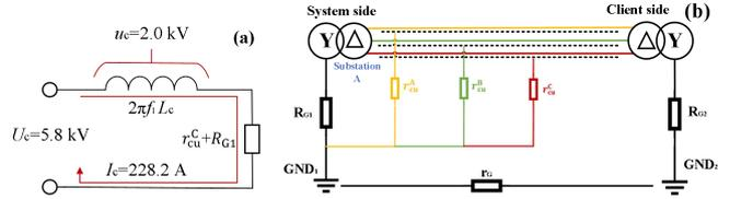
Fig.5 Equivalent electrical models at Stage 4 (a) Simplified equivalent circuit model of C phase, (b) Circuit topology diagram
