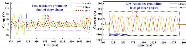
Fig.10 The voltage and current recording data at Stage 3
