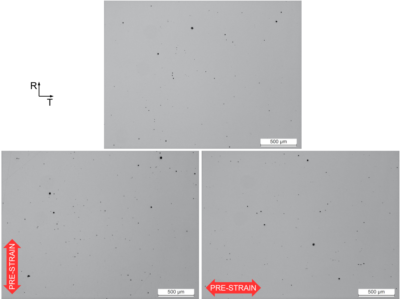
Figure 14: Optical microscopy of the DP600 before etching in both as received and pre-strained conditions
