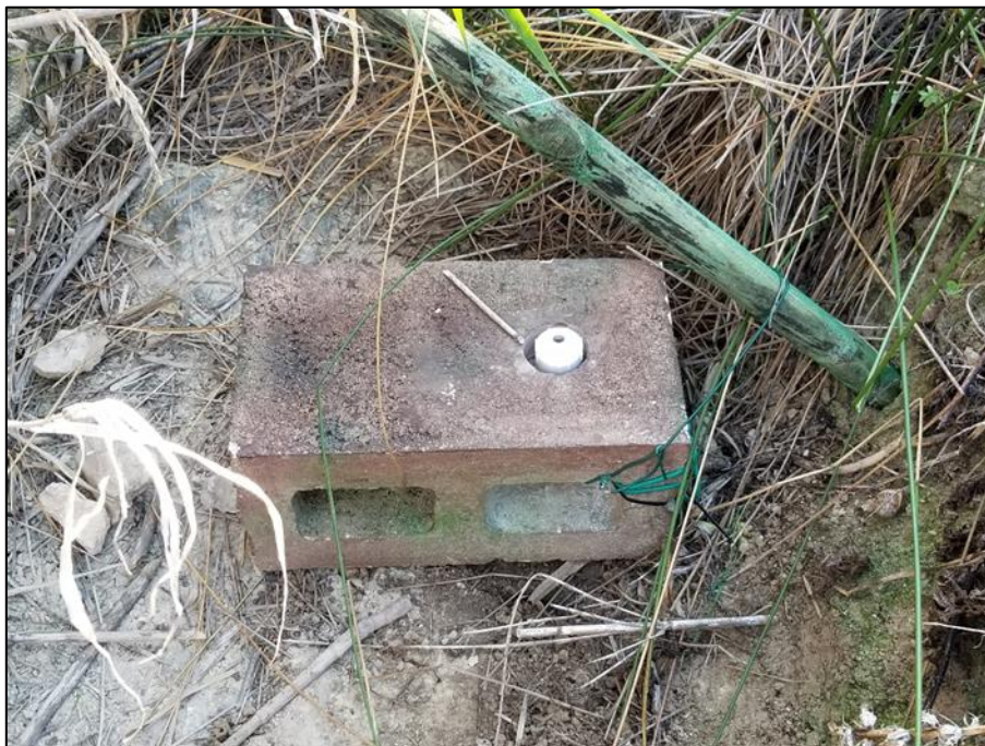
Figure 2. Onset HOBO U20L-04 with HOBO U2X Protective Housing deployed at Wied ta' Miġra l-Ferħa case study site.
