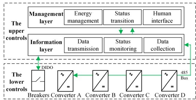
**Fig. 2.** The control frame of ER-MLFT.
