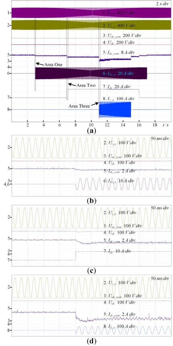
**Fig. 9.** The ER-MLFT experiment waveforms in Case B. (a) The voltages and currents. (b) The detailed waveforms of Area One. (c) The detailed waveforms of Area Two. (d) The detailed waveforms of Area Three.
