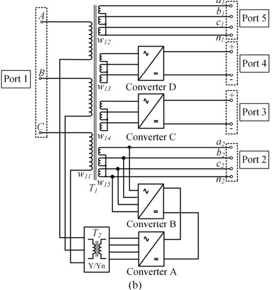
**Fig. 1.** The structure of ER-MLFT. (a) Energy subnet. (b) Main circuit topology.
