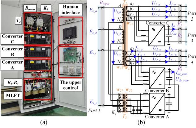
**Fig. 7.** The experimental prototype of ER-MLFT. (a) The experimental prototype. (b) The topology of the prototype.
