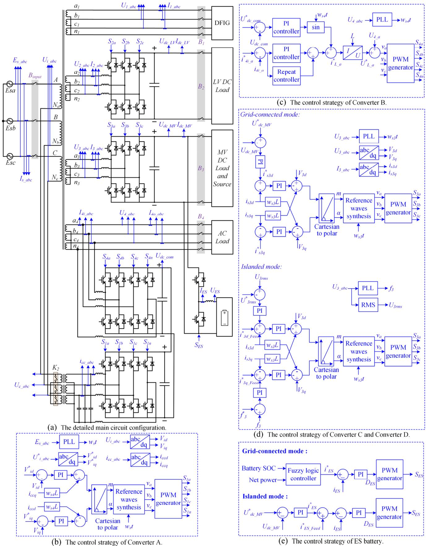
**Fig. 3.** The lower control strategy of ER-MLFT. (a) The detailed main circuit configuration. (b) The control strategy of Converter A. (c) The control strategy of Converter B. (d) The control strategy of Converter C and Converter D. (e) The control strategy of ES battery.
