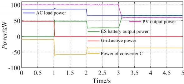
Fig. 4. The simulation waveforms of ER-MLFT in Case A.
