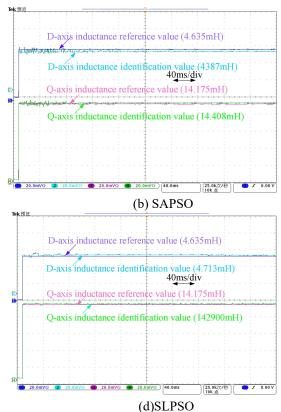
Fig. 9 shows the estimation curves of inductance by the four algorithms. Changes in working conditions and parameters cause the system to fluctuate. PSO is greatly affected, the parameter estimation accuracy of inductance is reduced by 4.2%, the accuracy of the optimized SAPSO, MTAPSO and SLPSO are reduced by 1.95%, 0.45% and 0.39% respectively. The accuracy of SLPSO decreases relatively lower, and its error remains within 2%.
