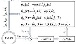
Fig. 2 Block diagram of parameter identification
