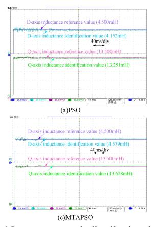
**Fig.6.** Parameter estimation results of  $L_d$  and  $L_q$  under condition 1.
