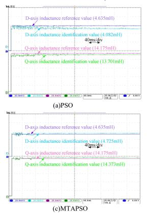
**Fig.9.** Parameter estimation results of  $L_d$  and  $L_q$  under condition 2.
