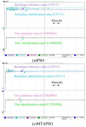
**Fig.5.** Parameter estimation results of R and  $\psi_m$  under condition 1.
