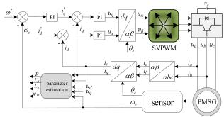
Fig.3 Vector control system block diagram
