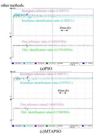
**Fig.8.** Parameter estimation results of *R* and  $\psi_m$  under condition 2.
