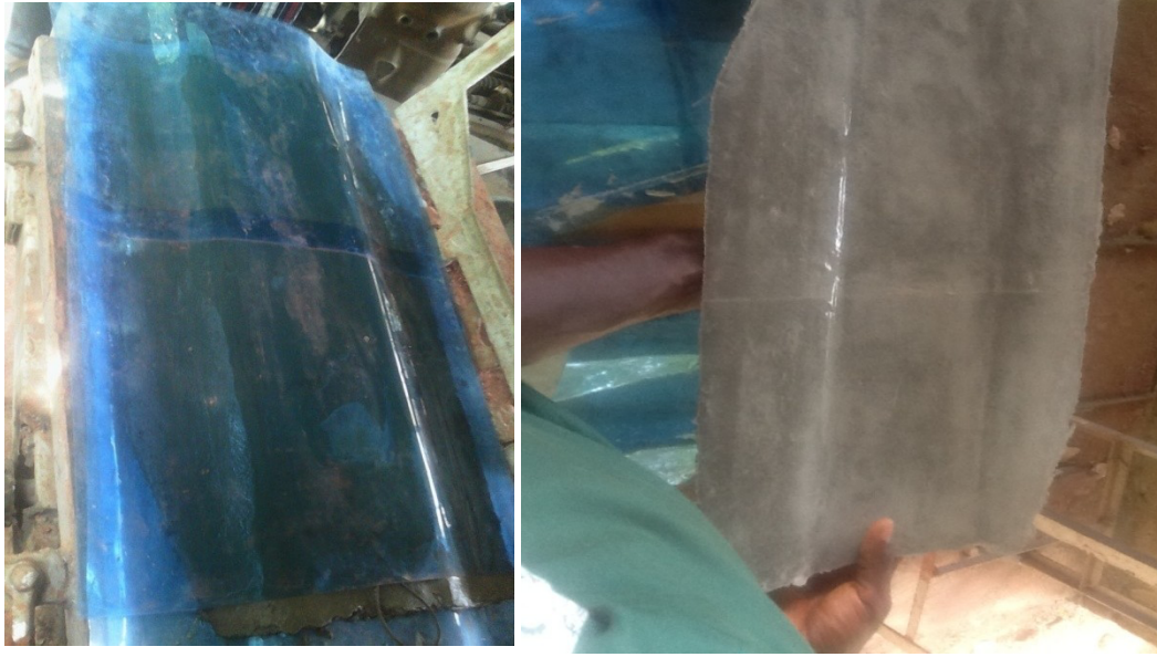
Plate 1: Slurry on corrugated mould Plate 2: Roofing tiles produced Covered with polythene ready for drying.
