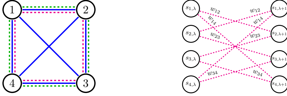
Figure 4 Compact representation of the coupling scheme for the traveling salesman problem. The blue and green couplings are the same as in Fig. 3. The magenta coupling is explicitly illustrated on the right side of the figure.
