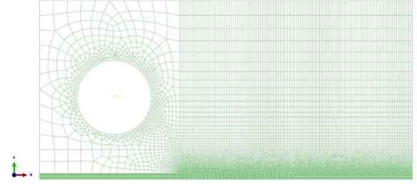
(a) Mesh of CT specimen
