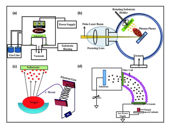
Figure: 2.4 Schematic Diagram of Physical Vapour Deposition
