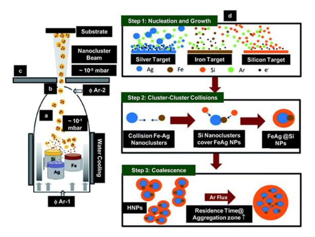
**Figure: 2.3 Inert Gas Condensation**
