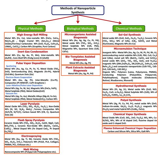
Figure: 2.1 Methods of nanoparticles synthesis
