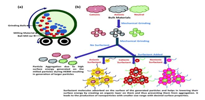
Figure: 2.2 High Energy Ball Milling Techniques
