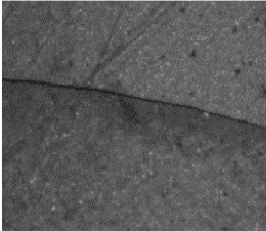
Fig. 2 Analysis of surface defects of  $\text{Si}_3\text{N}_4$  ceramic bearings roller inner ring
