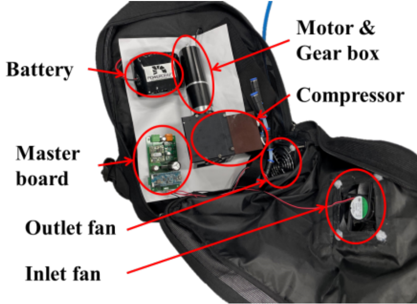
Fig. 4 Distribution of the actuator system. High temperature from each component can be cooled by two cooling fans.
