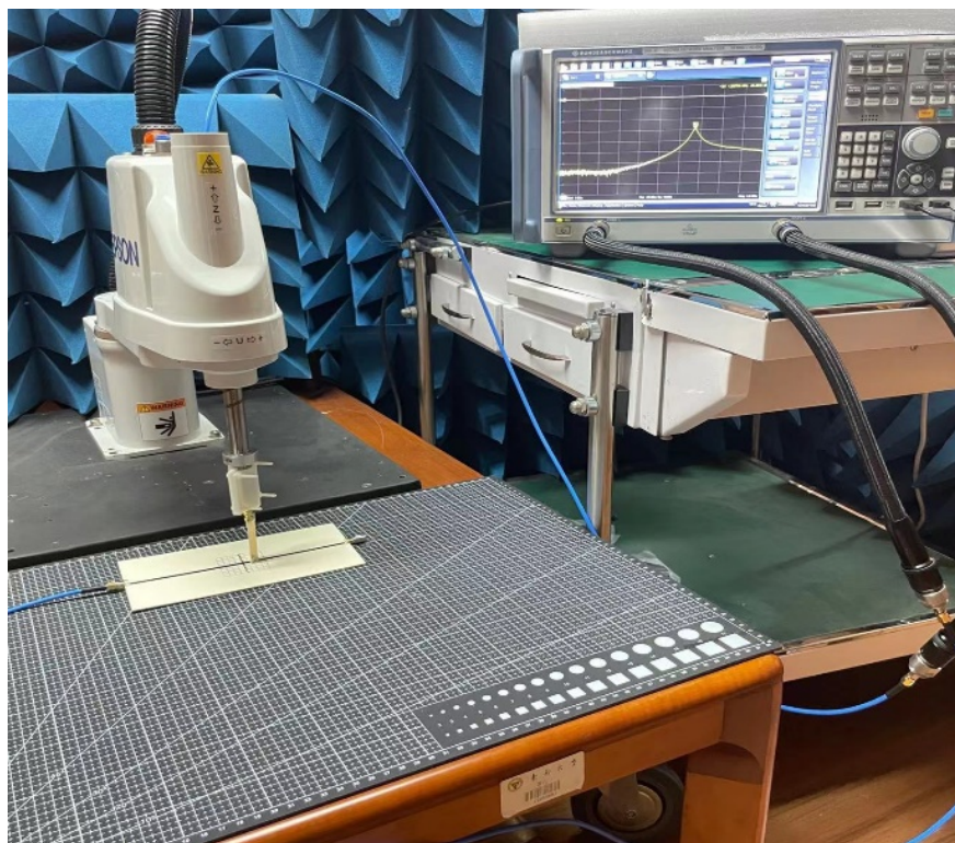
Fig. 5(b) The measurement setup of the probe
