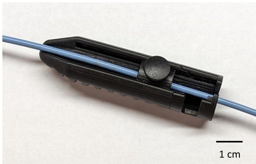
Figure 1: Catheter torque tool accessory designed with sliding sled to securely attach to cardiac ablation catheters ranging in size from 3-9 French and providing a larger surface area to grip and maneuver catheters. The tool is attached to a 7 French catheter as shown.
