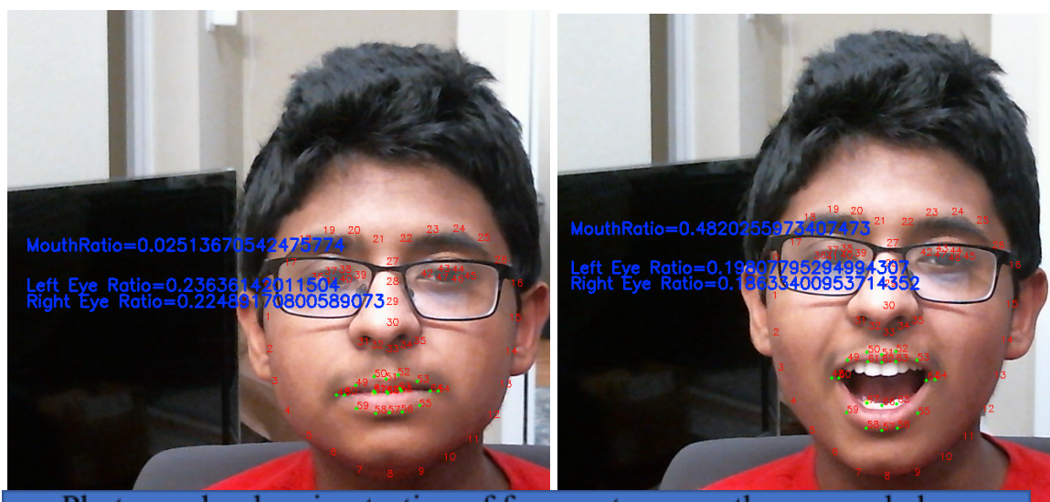
Photographs showing testing of face gesture mouth open and close detected by my algorithm and how the programmed ratios change
