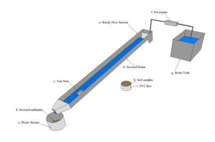
Fig.1. Schematic diagram of the experimental setup (Sun et al., 2018)
