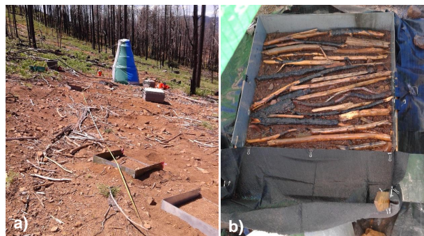
Figure 2. Portable rainfall simulator assembled over one plot on the skid trail, with wind-shelter in place (a) and detail of a compacted and slash-covered plot and the splash-collecting system (b).
