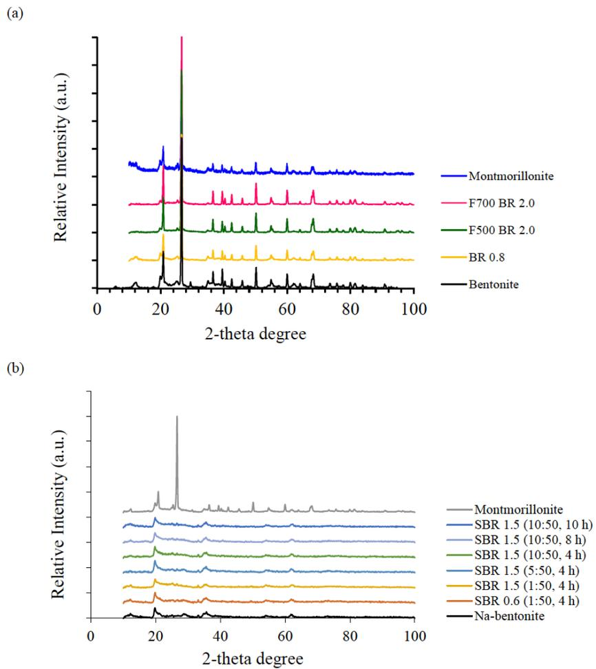
**Figure 1.** XRD patterns of (a) commercial clay, bentonite, and activated bentonites, and (b) Na-bentonite and activated Na-bentonites
