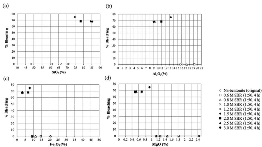
**Figure 3.** Relationship between % bleaching of palm oil and SiO<sub>2</sub> (a) Al<sub>2</sub>O<sub>3</sub> (b) Fe<sub>2</sub>O<sub>3</sub> (c) and MgO (d) contents of activated Na-bentonites.
