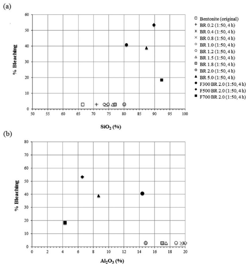
**Figure 2.** Relationship between % bleaching of palm oil and SiO<sub>2</sub> (a) Al<sub>2</sub>O<sub>3</sub> (b) contents of activated bentonites.
