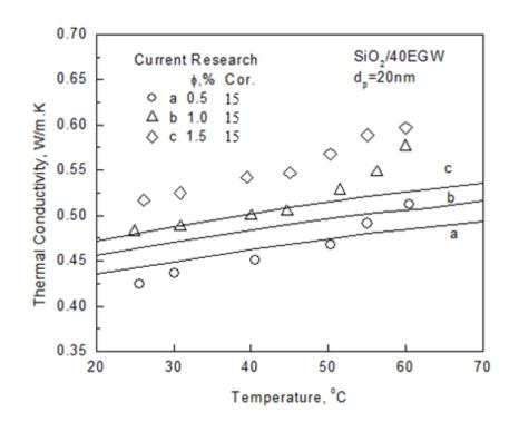
Figure 10 Comparison of experimental values of thermal conductivity for  $SiO_2/40EGW$  nanofluids with theoretical correlation (15)
