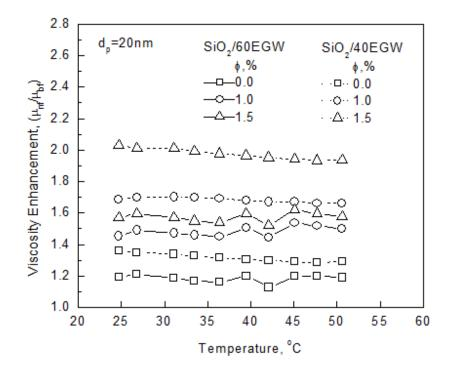
Figure 15 Comparison of viscosity enhancement of SiO<sub>2</sub>/60EGW and SiO<sub>2</sub>/40EGW nanofluids
