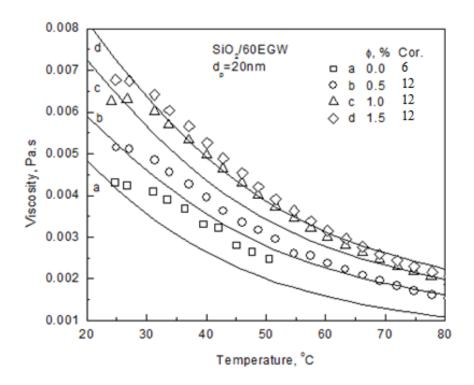
Figure 13 Comparison of experimental values of viscosity for  $SiO_2/60EGW$  nanofluids with theoretical correlations (6) and (12)
