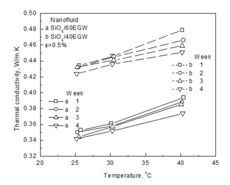
Figure 5. Thermal conductivity vs temperature weekly analysis
