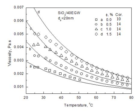
Figure 14 Comparison of experimental values of viscosity for  $SiO_2/40EGW$  nanofluids with theoretical correlations (10) and (14)
