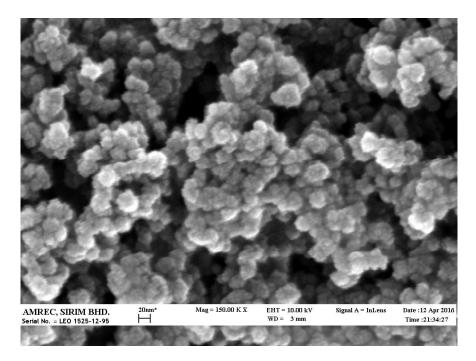
Figure 2 SEM Image of SiO<sub>2</sub> Nanoparticles
