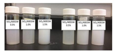
Figure 7: Nanofluid samples after one month of preparation
