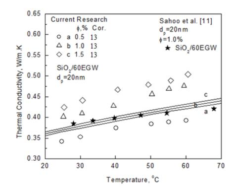
Figure 9 Comparison of experimental values of thermal conductivity for  $SiO_2/60EGW$  nanofluids with theoretical equation (14)
