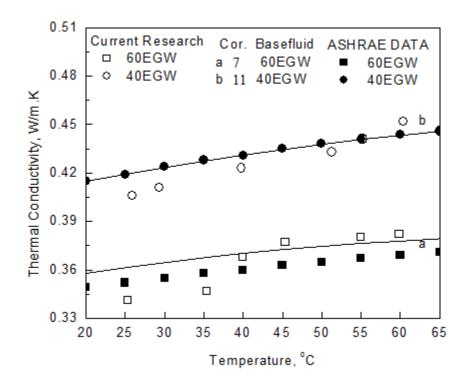
Figure 8 Comparison of experimental thermal conductivity values of base fluids with ASHRAE data
