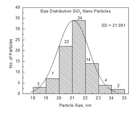
Figure 3: Particle Size Distribution of SiO<sub>2</sub> Nanoparticles
