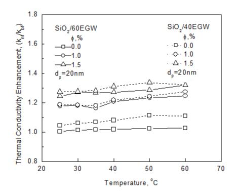
Figure 11 Comparison of thermal conductivity enhancement of  $SiO_2/60EGW$  and  $SiO_2/40EGW$  nanofluids
