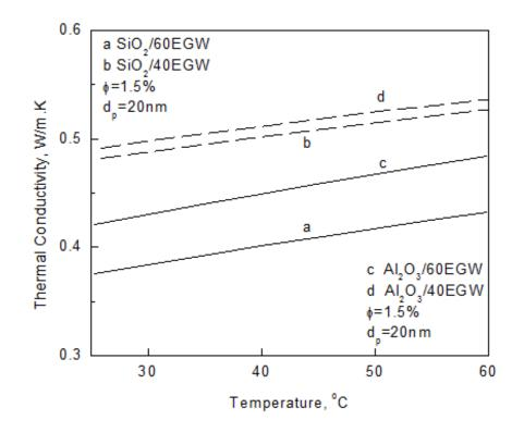
Figure 12 Comparison of theoretical thermal conductivity values for two different nanofluids
