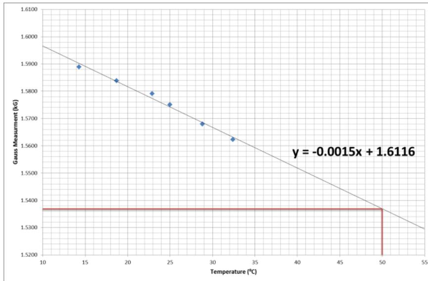
Figure 9 - Magnetic Field Strength (kG) vs Temperature (°C) - EXTRAPOLATED
