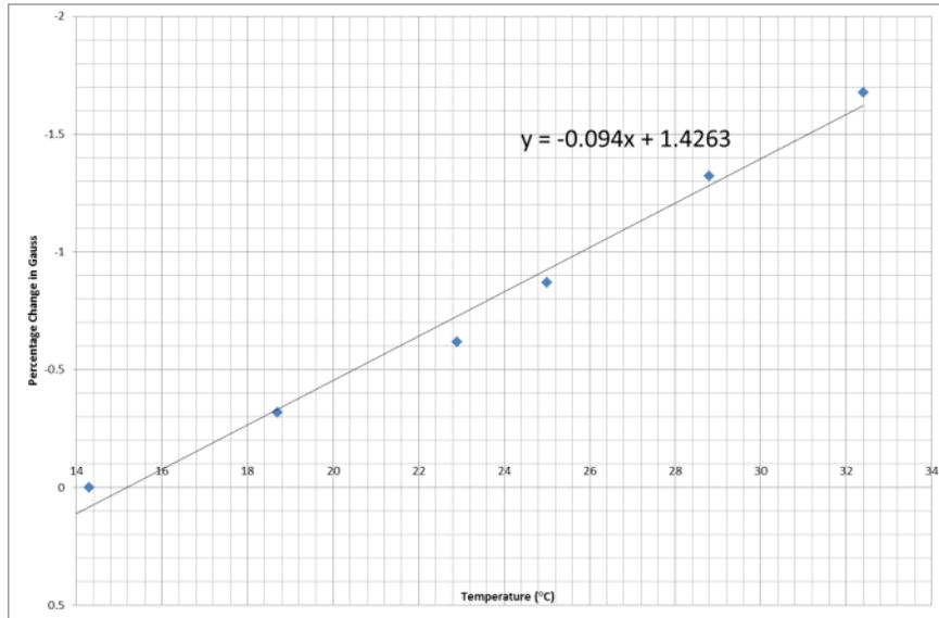
Figure 6 – Percentage Change in Magnetic Field Strength Reading vs Temperature (°C)
