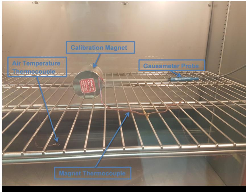
Figure 3: Experimental test set up 3
