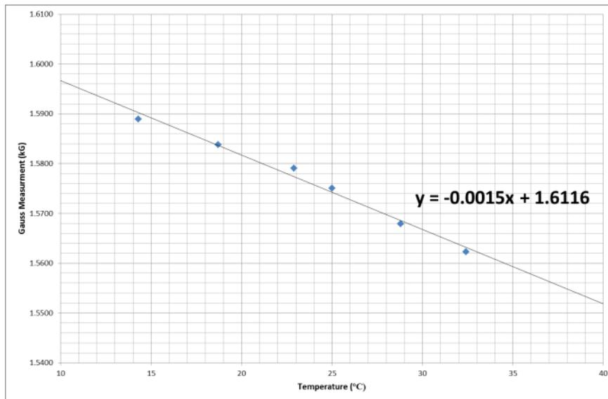
Figure 5 – Magnetic Field Strength (kG) vs Temperature (°C)
