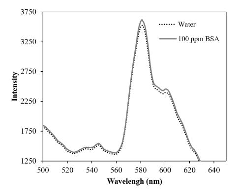
Figure 5 Fluorescence emission spectra of the Di-CHODPP in contact with Milli-Q water (black dots), and in contact with a 100 mg  $L^{-1}$  BSA solution (gray line).
