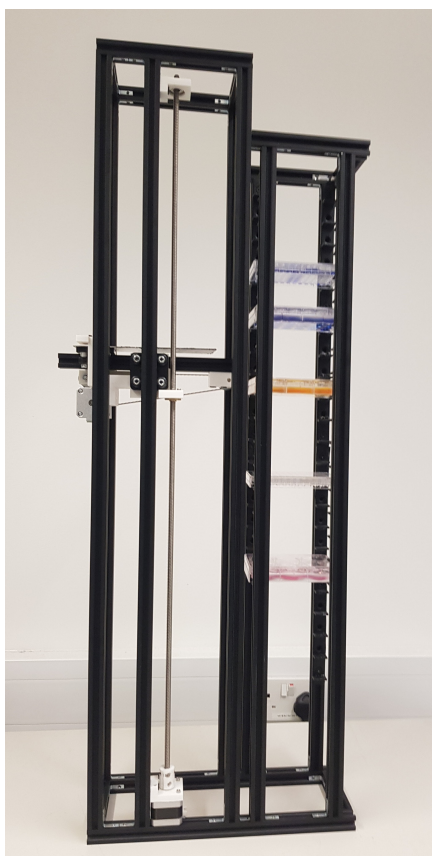
Figure 2: Photograph of a customised version of the apparatus. Note that in this design there is an open area above the stack of plates where the plate can be presented to other robotic devices which require space for access.
