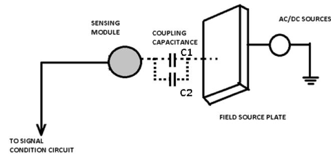
Figure 1: Schematic figure of the non-contacting measurement device
