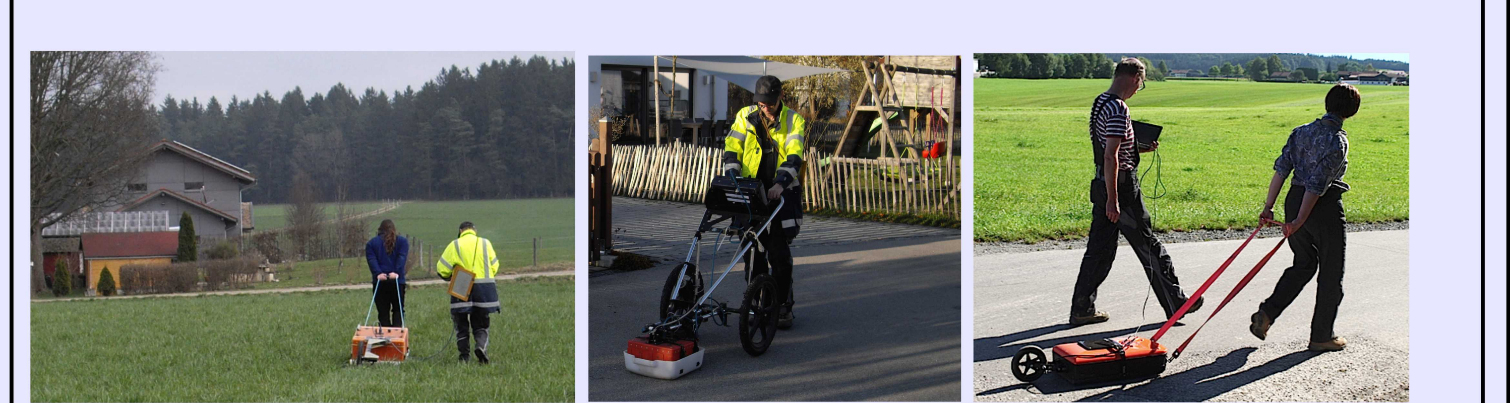
Thunderhole field work with ground penetrating radar (GPR) equipments: GSSI 200 MHz and 400 MHz, VIY3 300 MHz.
