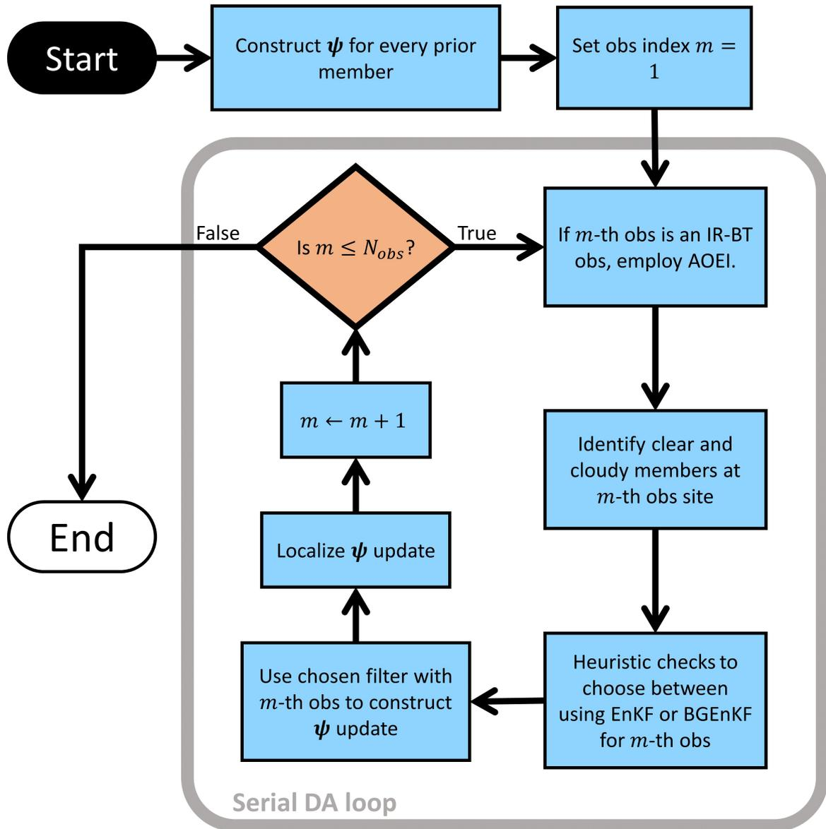
**Figure S2:** Workflow of the BGENKF module implemented in the PSU DA system. “Obs” stands for “observations” and  $N_{obs}$  stands for the total number of observations. See the text for the definitions of the extended state vector  $\psi$  [Eq. (3)], the list of heuristic checks used to select between the EnKF and BGENKF (main text section 2.5), and for a description of the BGENKF update procedure (Text S4). The three-stage BGENKF update procedure is illustrated in Figure 1 of the main text.
