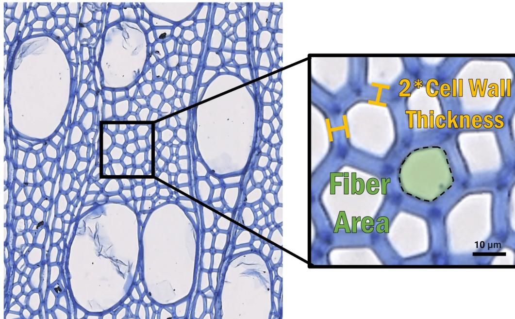
To better characterize these anomalous rings we used an approach known as quantitative wood anatomy (QWA). This technique identifies and measures each individual cell that comprises a tree ring. Measurements, as shown in the above figure, include the lumen area (LA) and cell wall thickness (CWT) of wood fibers cells.
